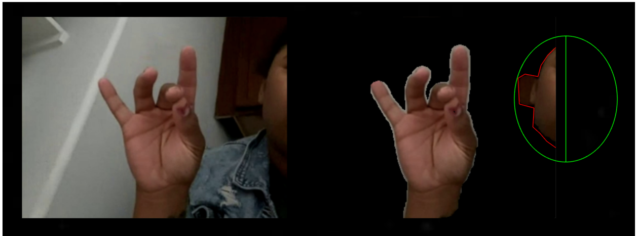
Figure: Showing masking output, hull lines, and the enclosing ellipse, which the hull lines do not fit into half of (denoted by the red hull and pixels fitting within half the generated enclosing ellipse. Resized for illustrative purposes.
